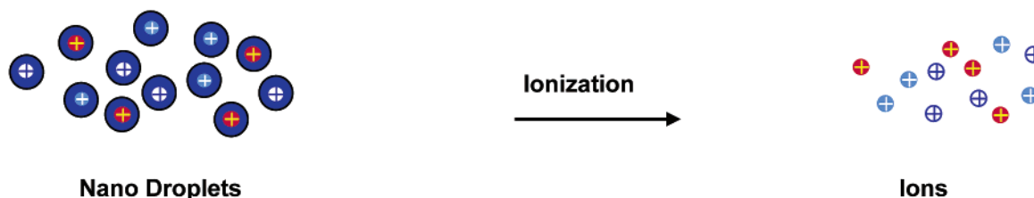
FIGURE 2. Simplified illustration showing concentration and flow rate effects on the ESI process. For larger flow rates, which produce larger droplets (Table 1), analyte surface activity, concentration, and competition from other species can affect overall ionization efficiency, the extent of ionization “suppression”, and quantitation. At sufficiently low flow rates and analyte concentrations, each droplet contains on average less than one analyte molecule, ionization efficiency is 100%, and suppression/matrix effects are eliminated.
